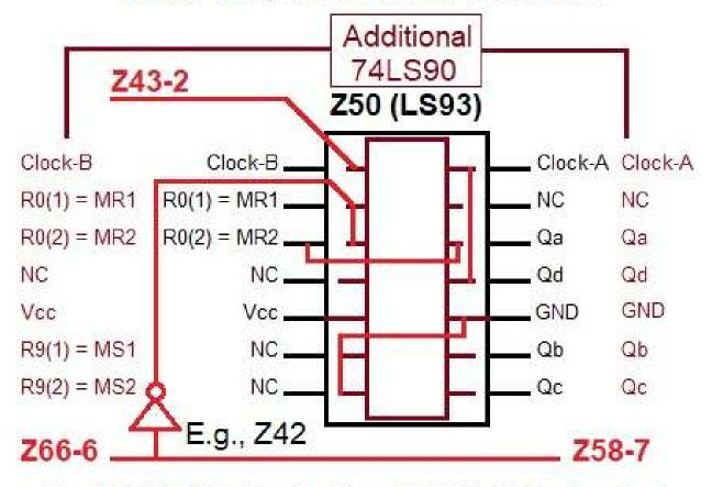
Cut LS92 Z58 pins 6+7 and LS93 Z50 pins 2+3
