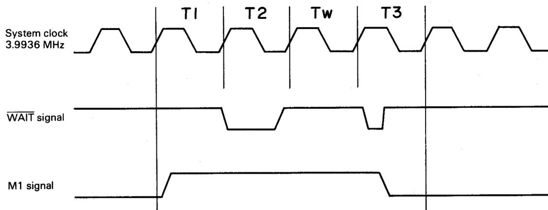
Fig. 4-15 M1 cycle with TW cycle (At 4 cycles)
