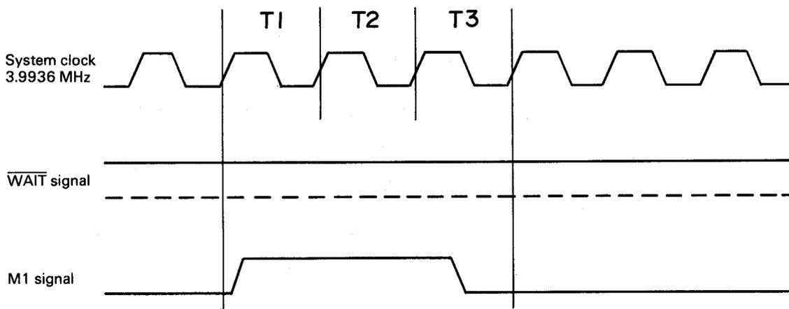
Fig. 4-14 M1 timing without TW cycle (At 3 cycles)
