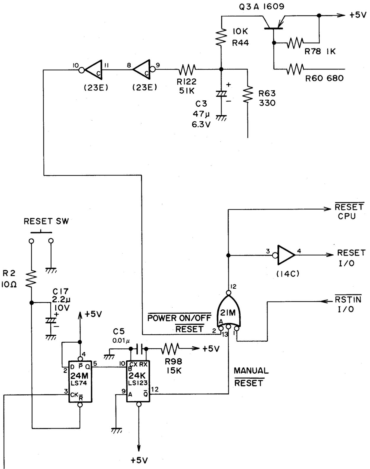
Fig. 4-1 Reset circuit
