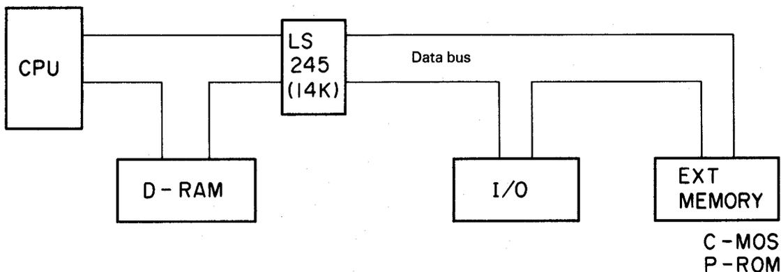
Fig. 4-11 Data bus line and peripheral devices
