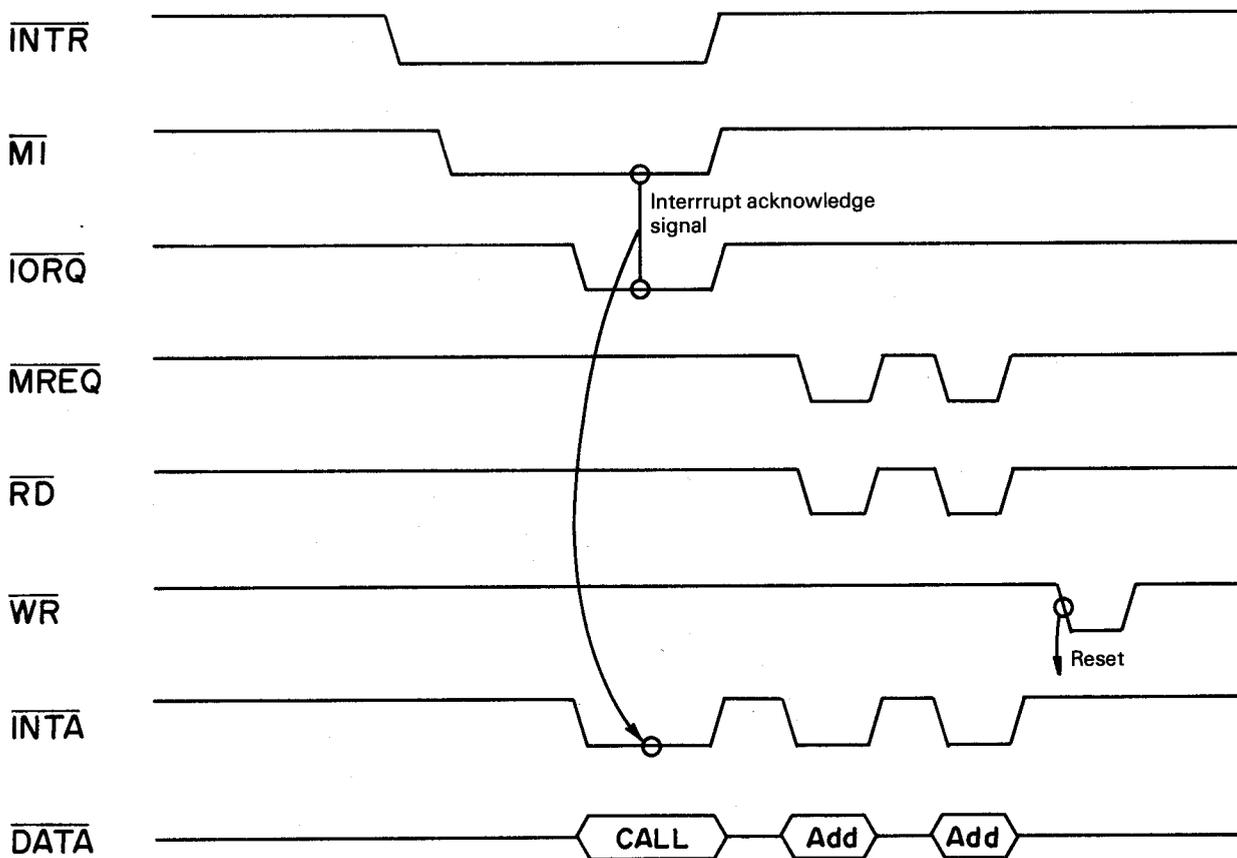
Fig. 4-8 Interrupt acknowledge signal timing
