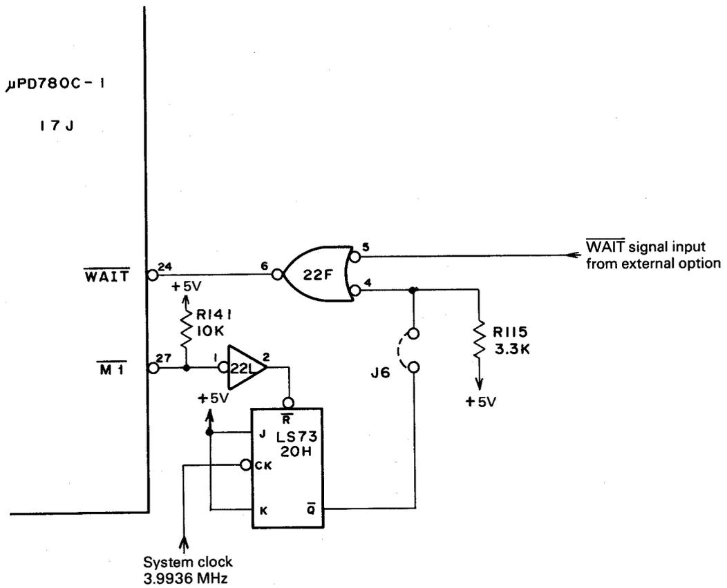
Fig. 4-16 WAIT signal supply circuit
