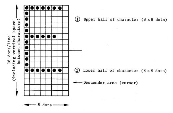
Since an  $8 \times 16$  dot pattern cannot be displayed in one operation,  $8 \times 8$  dot sections 1 and 2 are displayed in sequence by two operations.
