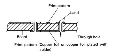
Fig. 6-7 Section of Board
