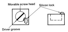
Fig. 6-8 Variable Resistor Locking
