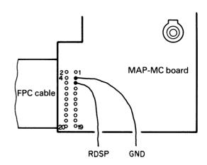
Fig. 6-18 Additional Lead Wires for Azimuth Adjustment
