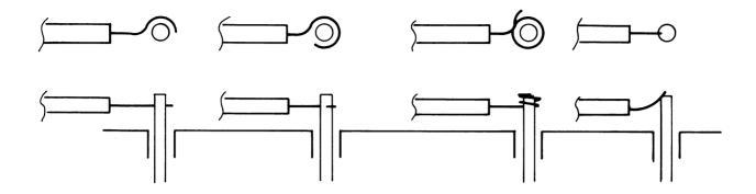
Fig. 6-5 Installing the Wire
