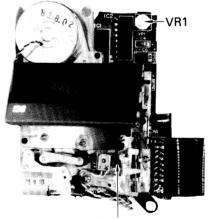
Azimuth adjustment screw (Located right beneath the azimuth hole cover.)
