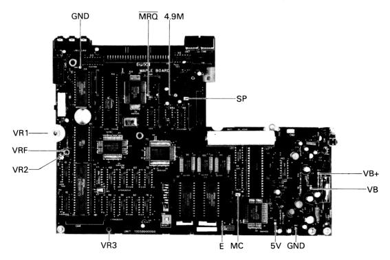
Fig. 6-13 MAPLE Board Variable Resistors
