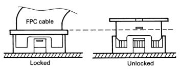
Fig. 6-10 FPC Cable Connection/ Disconnection
