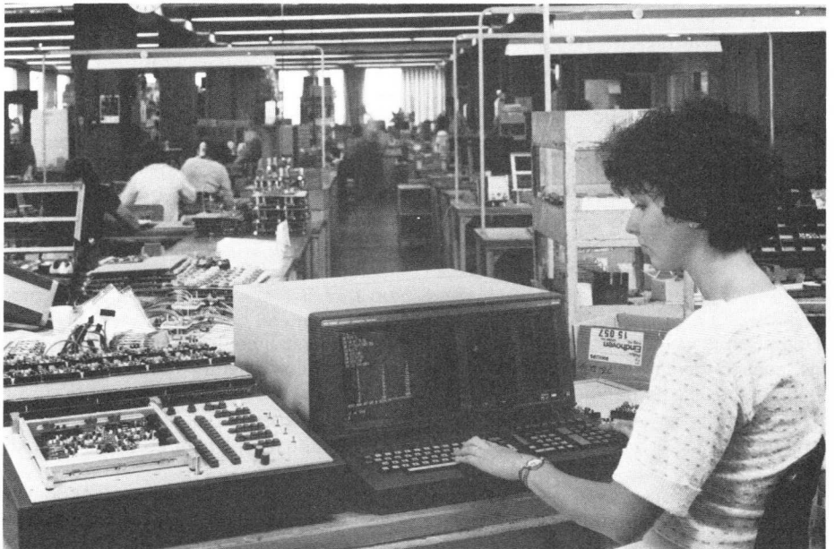
One line sample testing of component board using PM 4400.
