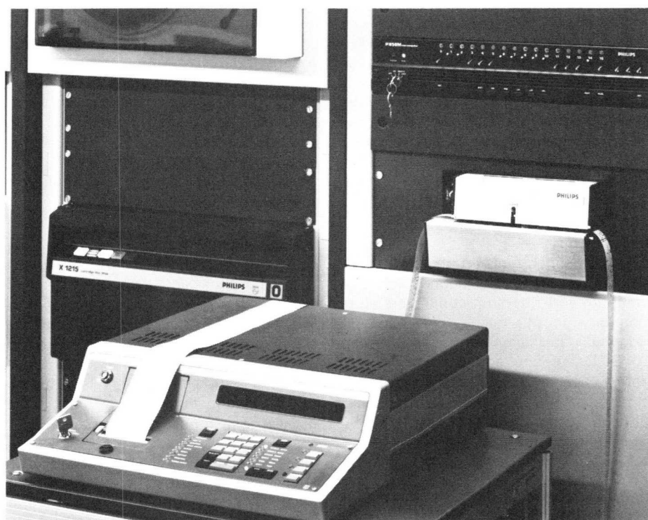
PM 4000 data logger operating in conjunction with a Philips P 800 series minicomputer.
