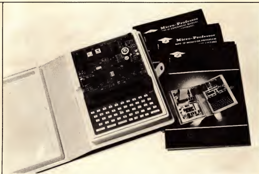
The MPF-1P Microprofessor. This is based on the Z-80 CPU, operates at 1.79 MHz and has on-board 4K RAM and 8K ROM. Other features are a 49-key keyboard, built-in speaker, interface for program storage/reading to and from cassette, 20-digit, 14-segment alphanumeric green tube display, 48 input/output lines, battery backup for the RAM contents, buss-expandable Z80 architecture and three user manuals.
