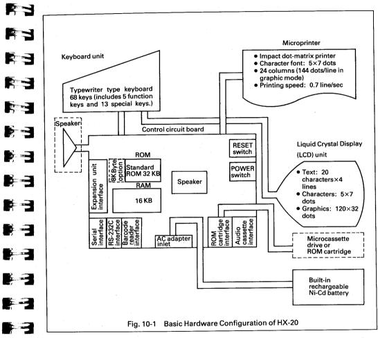
Your HX-20 comprises six major blocks as shown in the block diagram above; namely, a control circuit board, a keyboard unit, a microprinter, an LCD unit, a speaker, and a battery power supply. Each block is connected to the control circuit board and is neatly housed in the HX-20. The HX-20 is also equipped with an RS-232C interface, a serial interface and an expansion unit interface as standard equipment to permit system expansion through use of these interfaces.
