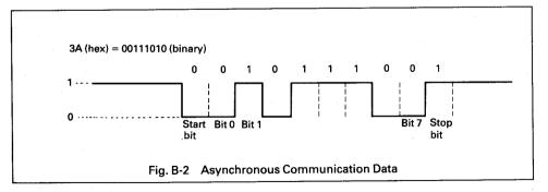
Actually, -8V (-3 to -15V) is output when the line level is "1" and +8V (+3 to +15V) is output when it is "0". Therefore, the relationship between the bit states and the line voltages is as shown below.
