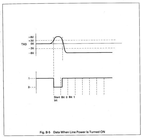
As a result, one incorrect bit may be received at the beginning of a data transmission when a programme list is serially output to the MX-80 by BASIC command LIST"COM0:". When programmes are transferred from one HX-20 to another (one using LIST"COM0:" and the other using LOAD"COM0:"), this incorrect bit can prevent the expected results from being obtained.
