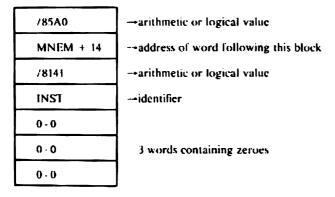
The parameter 16:14 indicates a word address seven words form the beginning of the expansion defined by FORM. The programmer has to specify this address as the last three words are left zero.
