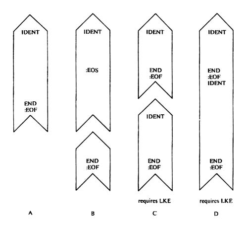
Example B is an example of a program punched on two tapes. The first tape starts with an IDENT and is terminated with :EOS which causes the Assembler to wait for operator action. The second tape does not contain an IDENT and is read immediately after the first one. The second tape is terminated by an END and :EOF.
