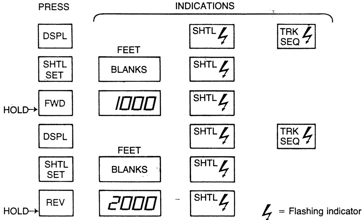
**NOTE:** If preset low tape BOT/EOT are set as shuttle points, the footage counter will display an L.
