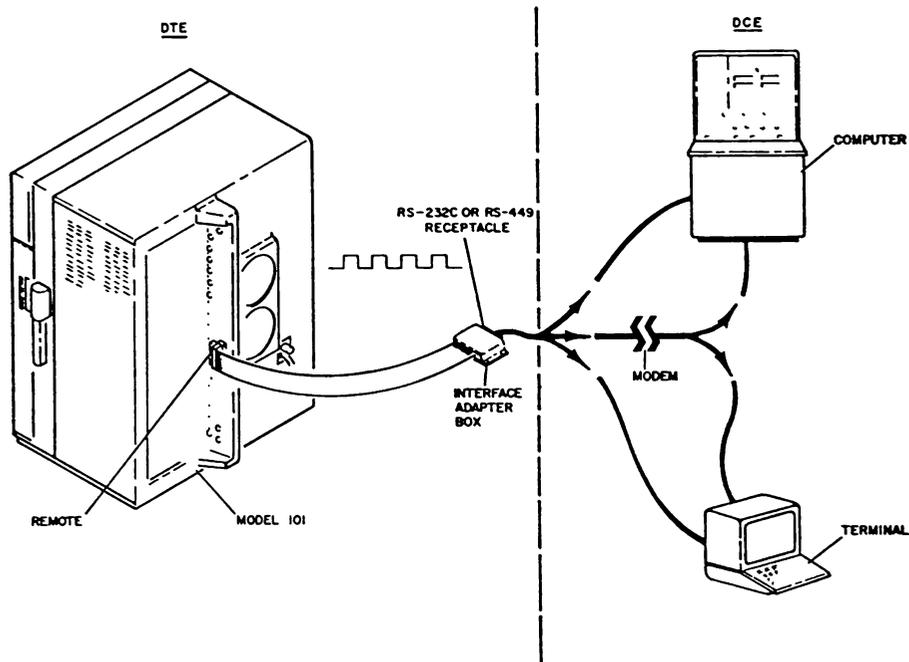
FIGURE A-1. RS-232C OR RS-449 BLOCK DIAGRAM
