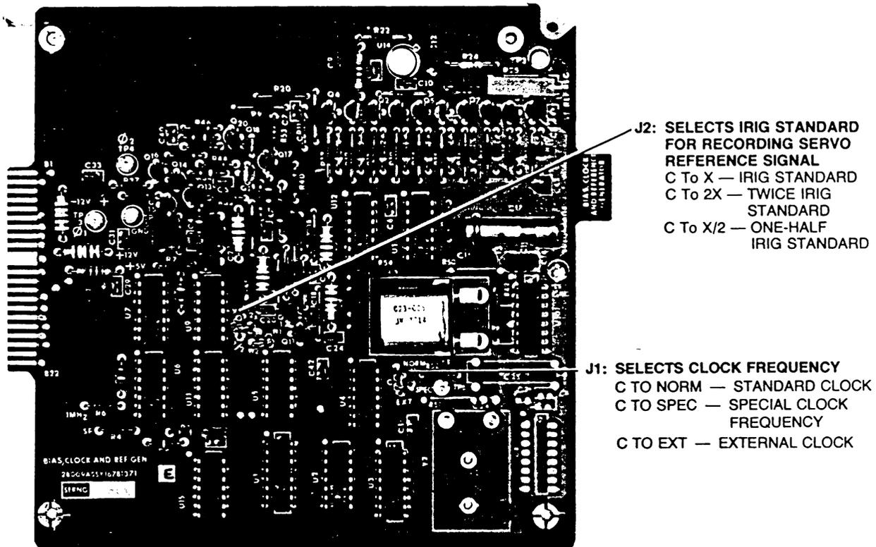
FIGURE 5-8. BIAS CLOCK AND REFERENCE GENERATOR CARD
