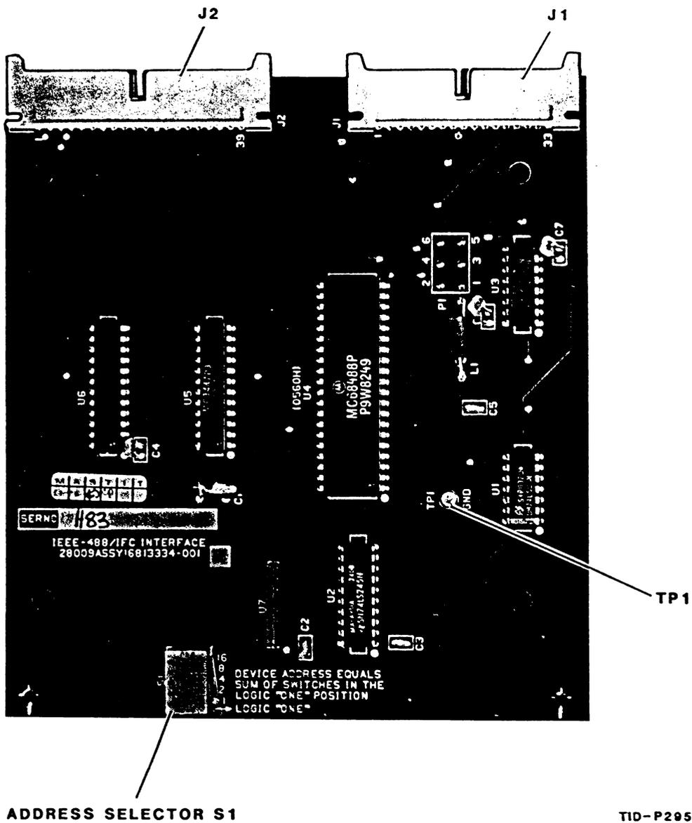
FIGURE B-3. 488 INTERFACE CIRCUIT CARD
