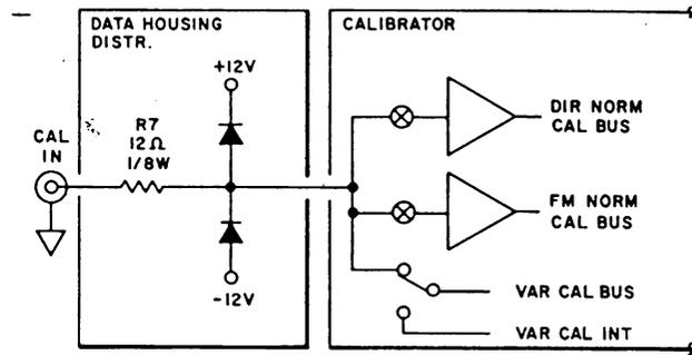
The external CAL signal should not exceed 10 volts peak or distortion will result. Higher signals may destroy R7 which provides circuit protection for the calibrator and record cards.
