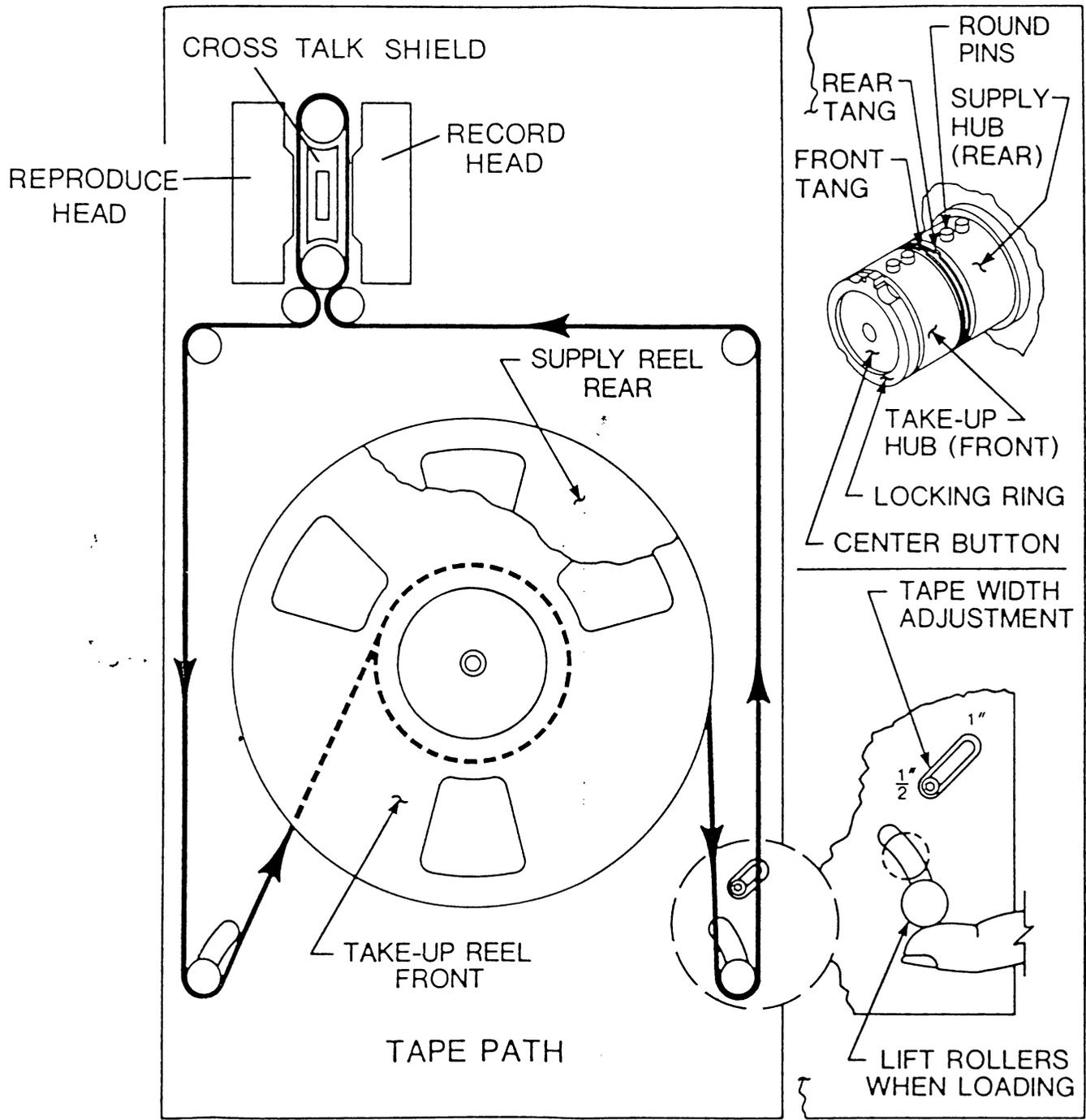
FIGURE 3-1. THREADING DIAGRAM
