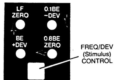
**LF/ZERO (Orange LED):** Indicates that a low frequency (LF) sinewave is applied to the variable cal bus if the **GAIN** indicator is lighted or the **DIRECT** normalize cal bus if the **DIR** indicator is lighted. If the **FM** indicator is lighted, the voltage on the FM normalized cal bus is the correct value to cause zero deviation of the FM carrier frequency.
