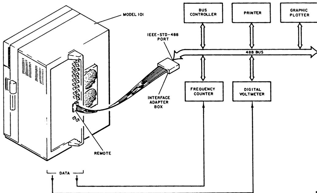
FIGURE B-1. MODEL 101/488 BUS SET UP — REPRODUCE MODE
