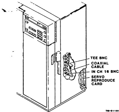
4. Connect the BNC TEE to the direct channel output BNC for channel being used for tape servoing. Extract data signal (mixed with carrier) from one side of the TEE. Connect a BNC cable from the other side of the TEE to the IN CH 16 (AUX IN CH 32 for auxiliary housing) on the Input/Output panel.
