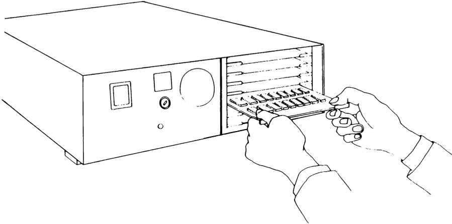
6. If an input/output option is being installed, remove the two screws holding the solid oval plate onto the card cage cover. After reinstalling the card cage cover, use the two screws to attach the shield plate supplied with the option, to the card cage cover. Affix the identification sticker to the outlined area on the card cage cover.
