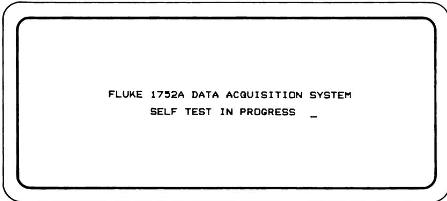
10. If the self-test is not successful, an error message is displayed on the screen. If this happens, recheck the previous steps. For a continuing failure, see the list of Self Test error messages in Section 3. If everything seems to be in order, perform the System Diagnostics as discussed in Appendix G. If further assistance is required, contact your Fluke Service Center.
