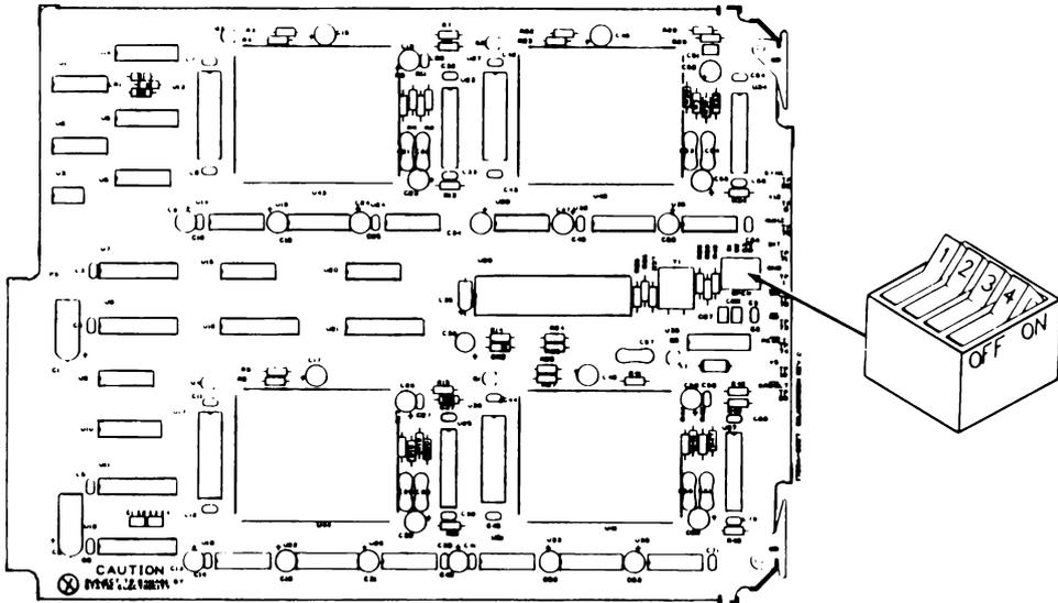
The 1752A has five slots available for options. Bubble Memory Modules can be installed in slots 1, 3, 4, 5 or 6. The SW1 address switch settings determine the device names, and the switch settings are identical for Option -004 (256K bytes) or Option -005 (512K bytes).
