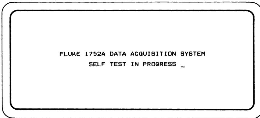
The benefit of this automatic test at power-up is that if it is successful, the 1752A's hardware is verified as operational, and if a problem occurs later, the hardware can be eliminated as the fault. If the test fails, press RESTART and try again. If the problem persists, contact your Fluke Customer Service Center.
