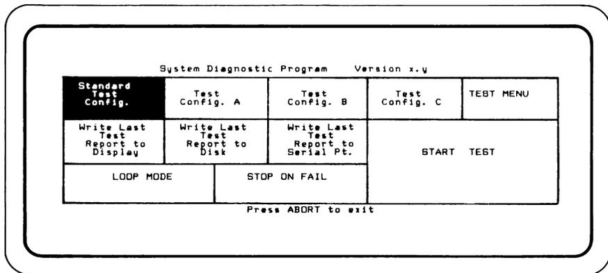
3. Touch the START TEST command block on the display to execute the Standard Test Configuration, or select individual tests as described in the following paragraphs.
