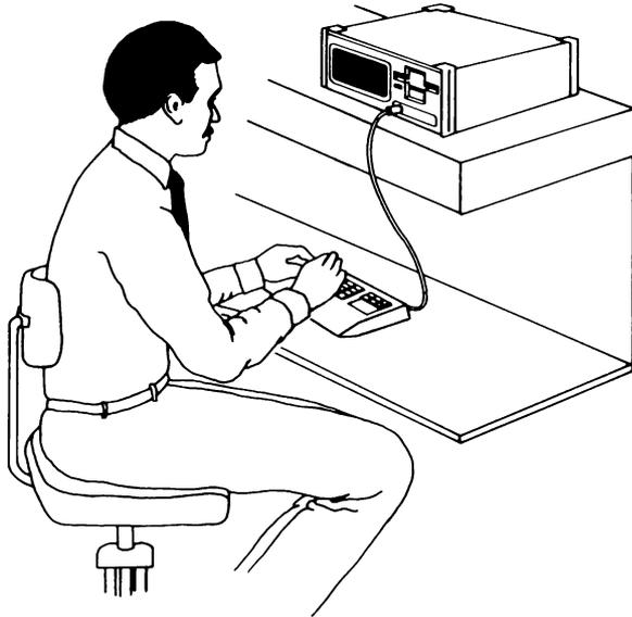
3. If instruments will be repeatedly connected and disconnected, make sure the back of the workbench is open and not against a wall. This makes connectors on the rear panel more easily accessible.
