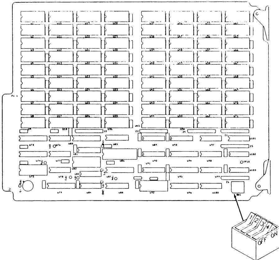
The 1752A has four slots available for options. Expansion memory modules can be installed into any or all of them. To assure proper operation of diagnostics software, the first module added should be given the address for Unit One as shown in the table below. Subsequently added modules are given addresses in ascending unit number order. The SW1 address switch settings shown below are identical for Option -006 (256K bytes) or Option -007 (512K bytes).
