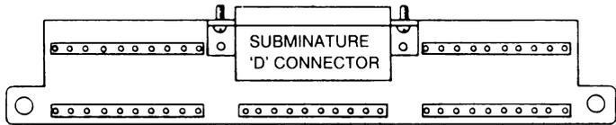
The 2400A-110 and 2400A-111 connectors provide numbered screw terminals or solder pins for convenient wire attachment. If only the female D-connector is used, external wiring must be soldered to the internal pins on the female connector.
