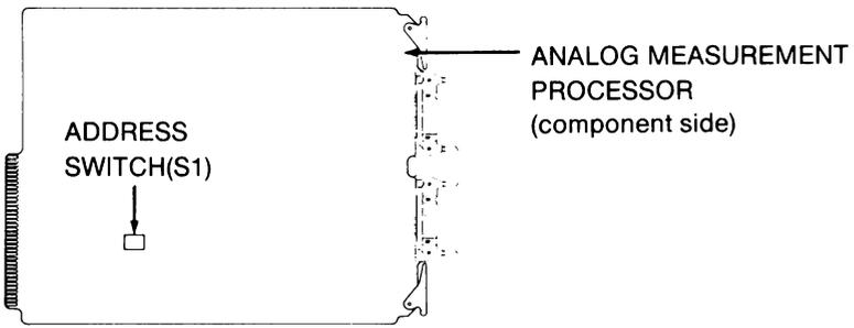
Note: Switch segment 1 is used for calibration, and should normally be OPEN.
