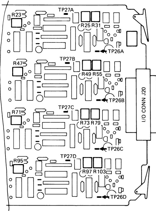
**ZERO TEST POINTS AND ADJUSTMENT POTENTIOMETERS**
