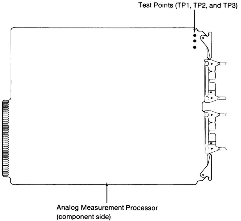
9. Place the DMM in the 2V range. Hook the + input lead of the DMM to TP1 and the - input lead to TP3. Using the 1752A keyboard, enter the reading of the DMM to the nearest  $\pm 10 \mu\text{V}$  following the 0.695V reference prompt.
