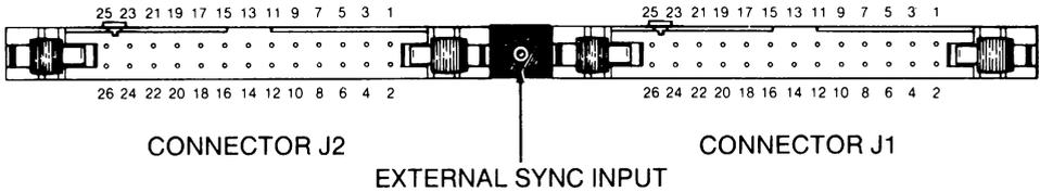
**INPUT CONNECTOR PIN ASSIGNMENTS**
