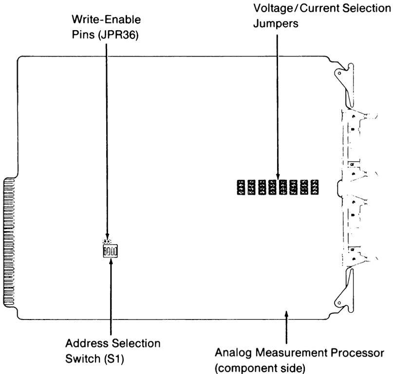
4. Place the Analog Measurement Processor back into the 1752A.
