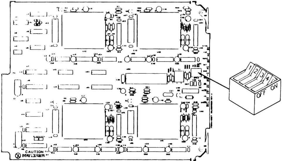
The 1722A has five slots available for options. Bubble Memory Modules can be installed into any three of them. The SW1 address switch settings determine the device names, and are identical for Option -004 (256K bytes) or Option -005 (512K bytes).
