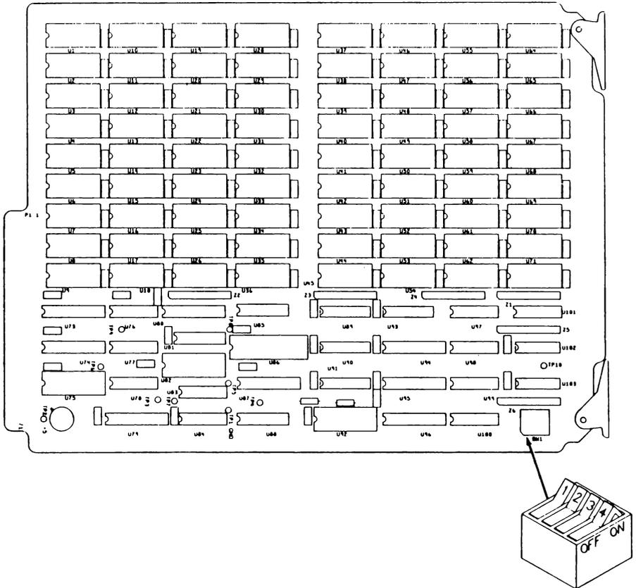
The 1722A has five slots available for options. Expansion memory modules can be installed into any or all of them. To assure proper operation of diagnostics, the first module added should be given the address for Unit One as shown in the table below. Subsequently added modules are given addresses in ascending unit number order. The SW1 address switch settings shown below are identical for Option -006 (256K bytes) or Option -007 (512K bytes).
