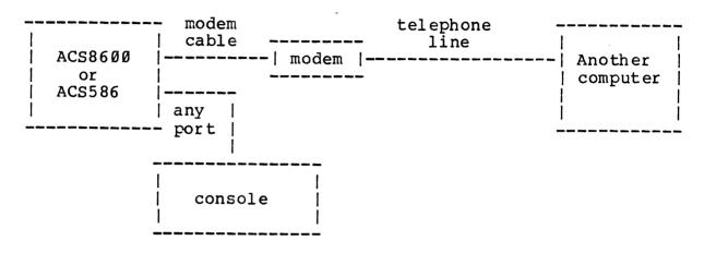
A special cable (usually called a "computer to modem" cable) must be used to attach a modem to either the 8600 or the 586. Most modem manufacturers and cable manufacturers supply these cables as off-the-shelf items. However, if the proper cable cannot be found, it may be necessary to build your own cable. To assist you, the RS-232C pins used by the 8600 and the 586 are shown below:
