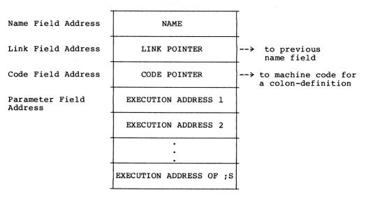
In this and all such diagrams in this manual, memory addresses increase from top to bottom.
