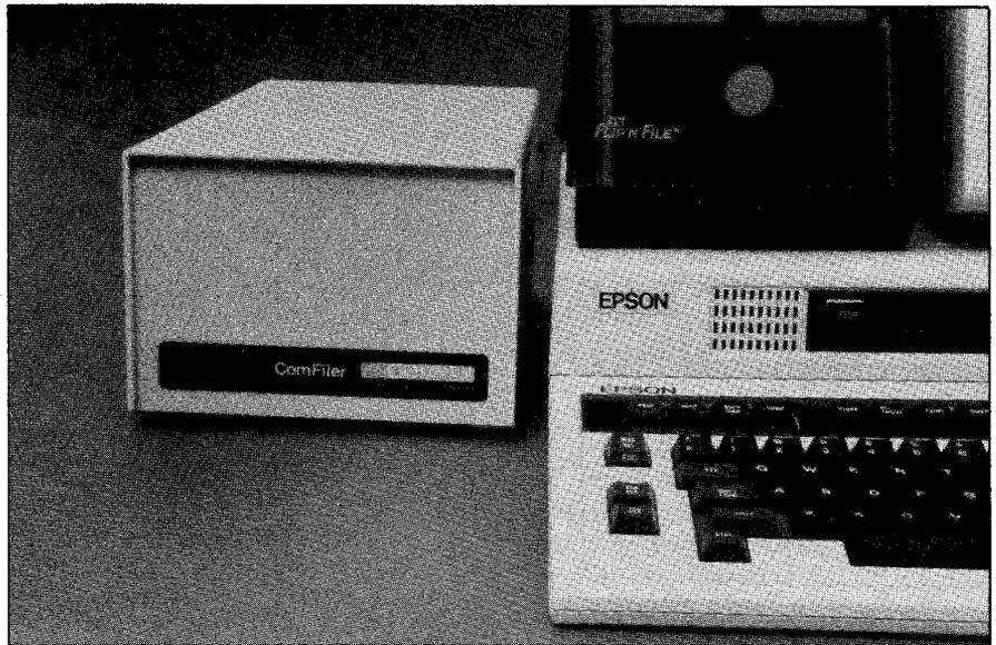
The Comrex ComFiler 10 megabyte hard disk. The ComFiler, although lower in capacity than most QCS hard disks, is slightly faster.
