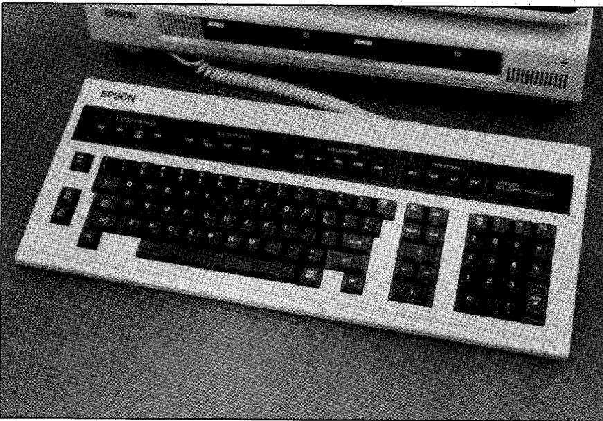
The HASCI-2 keyboard. Except for the edit key added to the applications area and the numeric sign inversion key to the calculator keypad, the layout is identical to the original keyboard.
