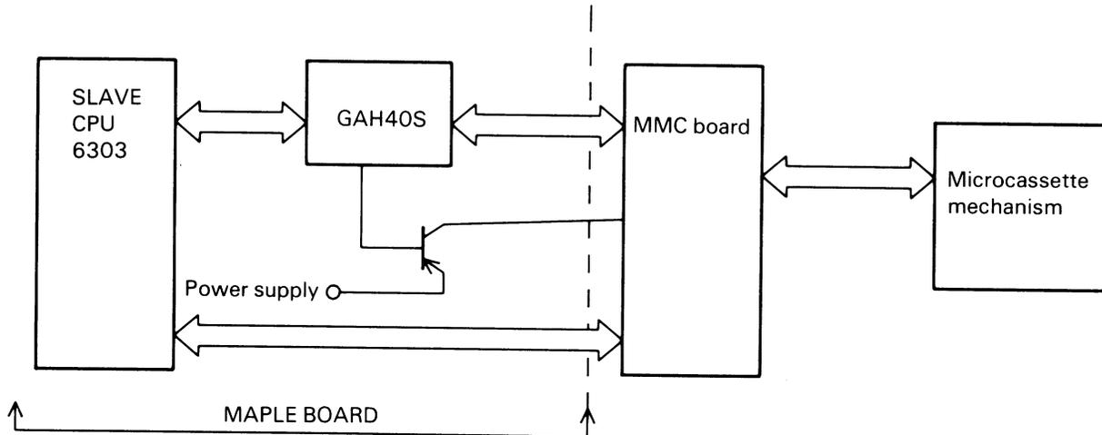
**Fig. 3-1 Microcassette Tape Operation Control Block Diagram**
