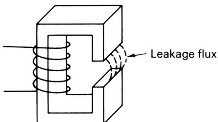
Data are actually written on the tape at the copre slit where leakage flux is generate.
