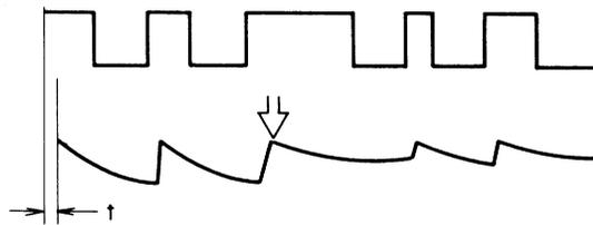
**Fig. 3-9 Integrating Circuit**
