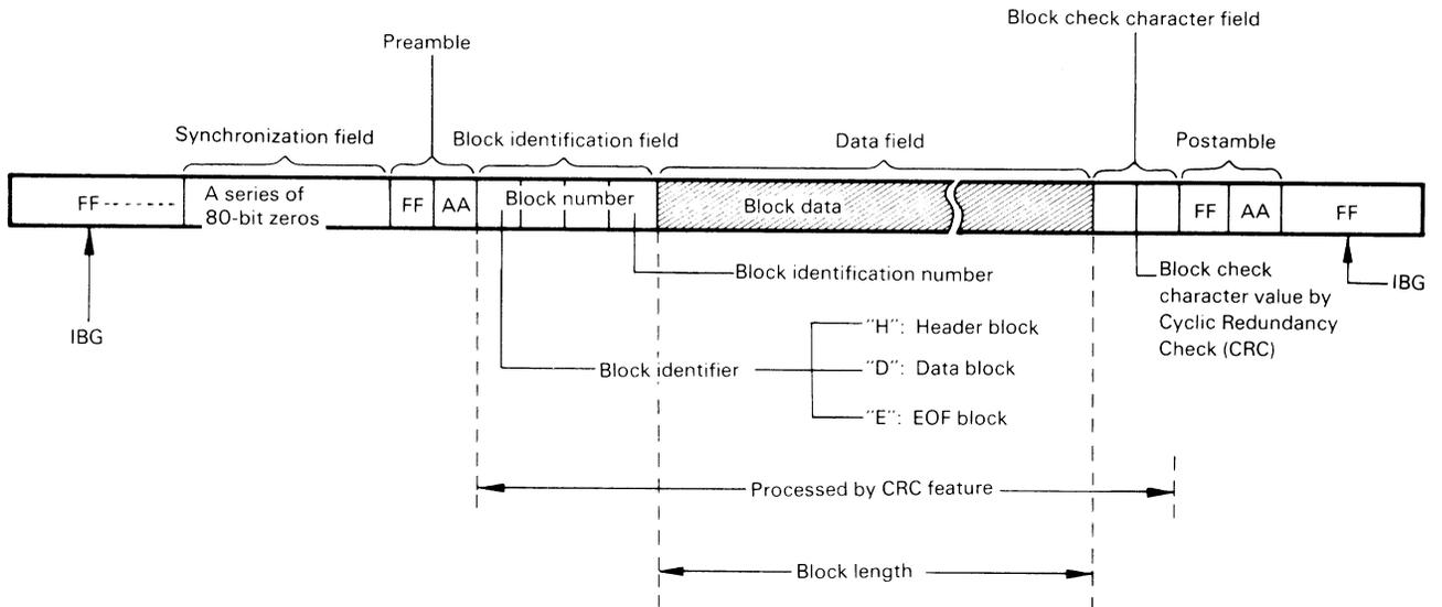
**Fig. 3-2 Microcassette Tape Data Format**
