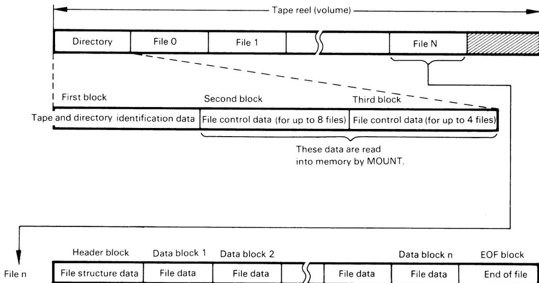
**Fig. 3-3 Cassette Tape Reel Structure**
