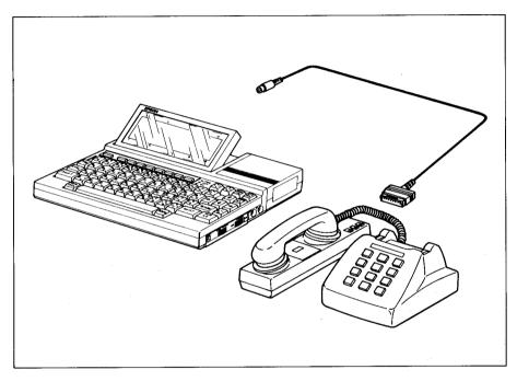
In addition to making it possible to communicate with other personal computers, the CX-21 allows PX-4 to be used as a remote terminal of any main frame computer system which can be accessed via the public telephone system. See the User's Manual for procedures for using the CX-21.
