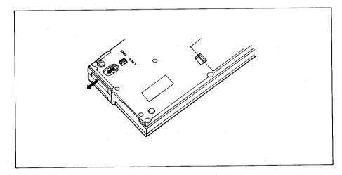
4. Next, place the cartridge to be installed in the cartridge slot so that its release ring fits into the hole in PX-4's bottom panel.
