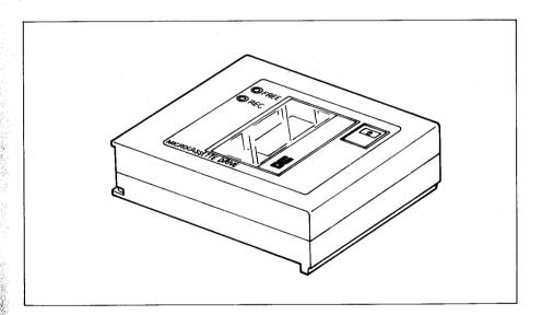
EJECT button: Press this button to remove tapes from the microcassette drive.
