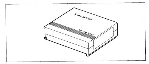
The RAM cartridge has a capacity of 16K bytes, and is accessed as drive I:. Before using the RAM cartridge, it must be formatted from the System Display. Ordinarily, formatting is a one-time process which does not need to be repeated as long as data inside the cartridge is not corrupted.
