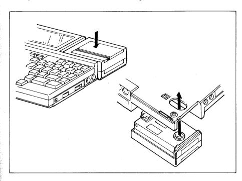
5. Push the cartridge in the direction indicated by the arrow to set it in place.
