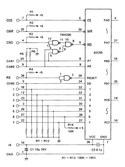
This example connects a 82C55 to the interface operating in the DB mode. If you make this circuit, be sure to check operation before use.
