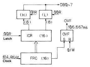
With the PINE, elapsed time is determined by latching the free running counter value in the input capture register. The FRC is continuously incremented by the system clock and the OVF flag is set to generate a main CPU interrupt when the counter overflows. The OVF flag is reset by the operating system.
