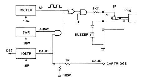
The PINE's speaker interface makes it possible to connect an external speaker or amplifier. The SP signal is switched for external output by inserting a plug into the speaker jack.
