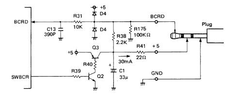
Power can be supplied to a device connected to the BCR jack by setting the SWBCR flag. This is shown in the figure above.
